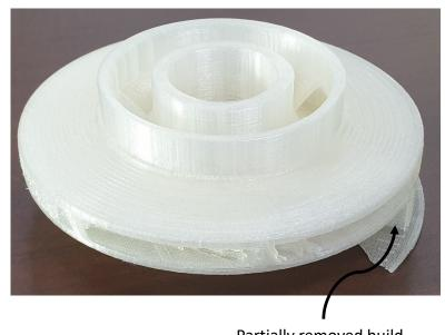
Partially removed build supports are shown
